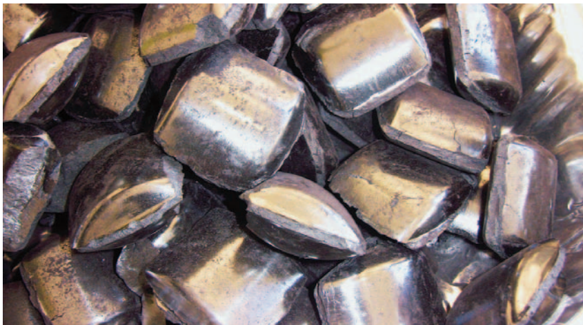
Using a proprietary binder, GreenFields produces a very durable briquette from fine coal.
